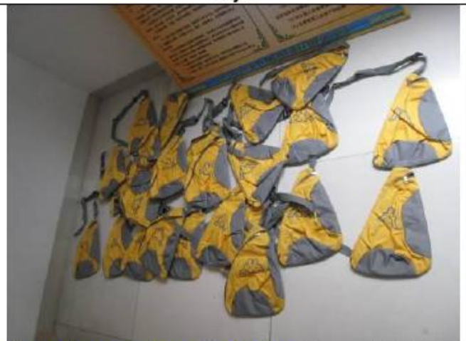
Defective samples collection for One end of strap detached or broken after pull test-travel bag--Major
