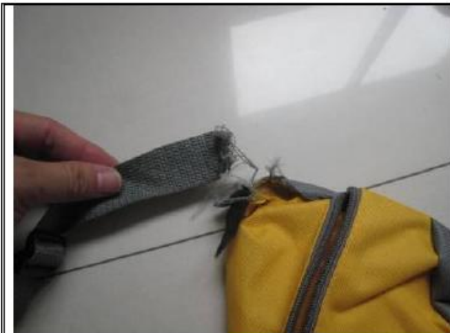
One end of strap detached or broken after pull test-Major
