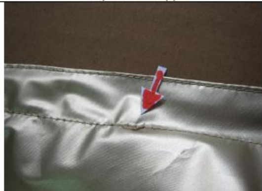
Top Panel View (6)-Messy Stitches-Minor Defect-1PC
