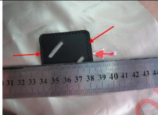
Remark #1- For all inspected samples, found visible uneven stitches along the 4 edges of patch (2).
