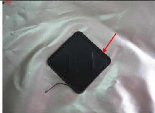
Remark #1- For all inspected samples, found visible uneven stitches along the 4 edges of patch. (6)
