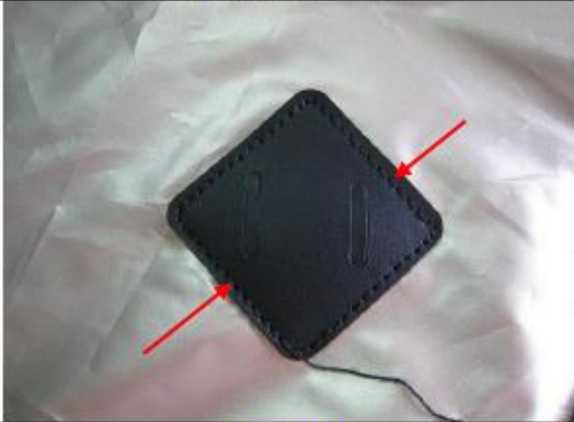
Remark #1- For all inspected samples, found visible uneven stitches along the 4 edges of patch. (3)
