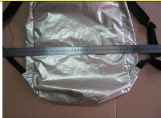
High-Low Side Panel-Major Defect (2)
