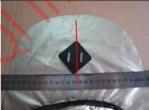
Remark #2- Slight Off Center For patch-5PCS Out of 32PCS-Major Defect
