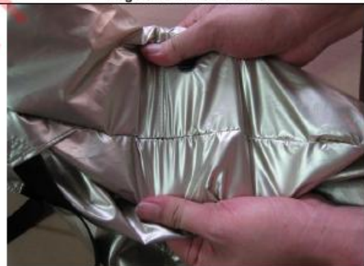
Pull Test for Seam by Hand force-Found OK After Test
