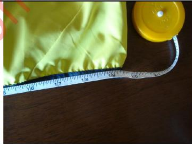
Size check on bottom of CH size(required is 18",actual size is 19.5")
