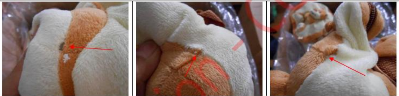
Broken holes -Major
