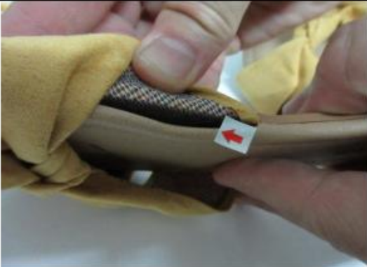
Outstanding Lack of glue inside(Major Defect)
