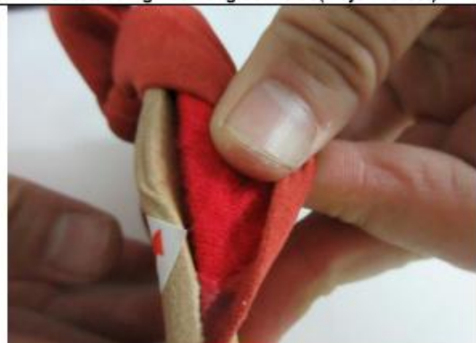
Outstanding Lack of glue inside(Major Defect)
