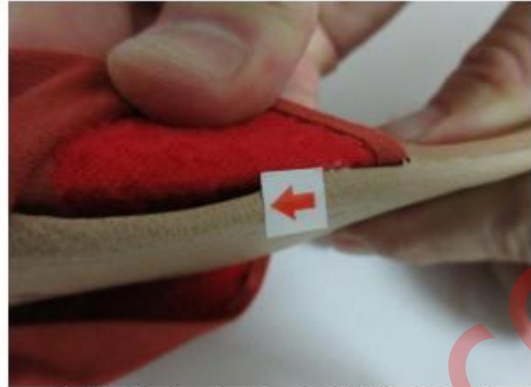
Outstanding Lack of glue inside(Major Defect)
