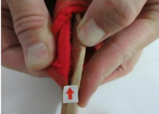
Outstanding Lack of glue inside(Major Defect)
