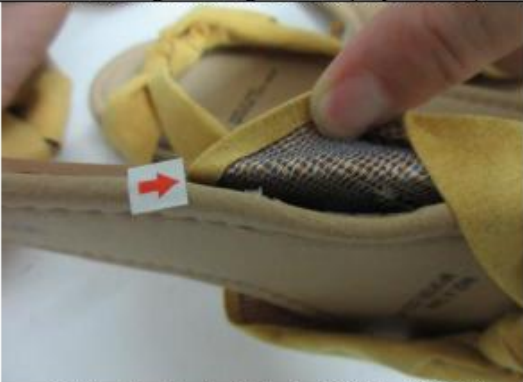
Outstanding Lack of glue inside(Major Defect)
