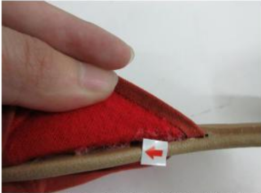
Outstanding Lack of glue inside(Major Defect)
