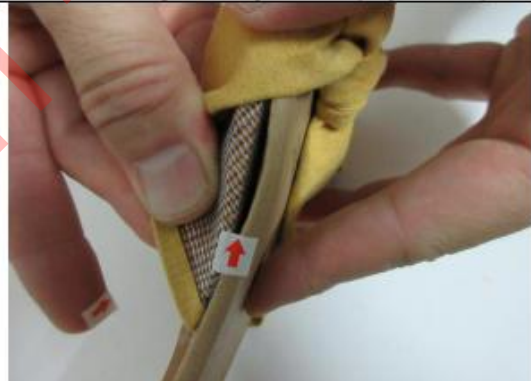
Outstanding Lack of glue inside(Major Defect)
