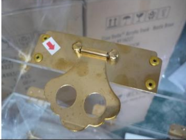
Remark 3: Found all the surfaces of rustic copper hardware oxidized.
