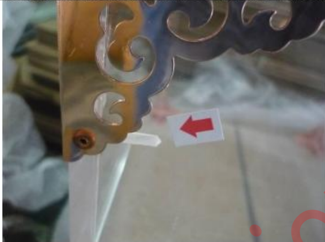
Remark 4: Found 30% of sample size for rustic copper hardware and rose gold hardware had white marks were showed inside, the factory explained they were caused when workers punched the screw holes, which made the holes too deep.
