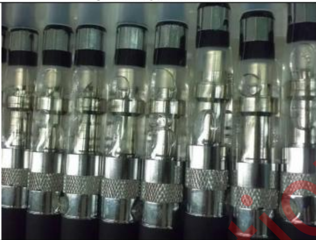
Waiting for 4H check for liquid leakage
