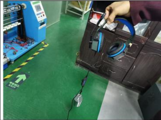
Cable pull test
