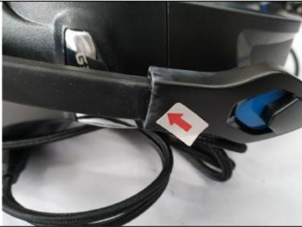
Remark 1: Found 75pcs with white mark on product, which was cleanable.
