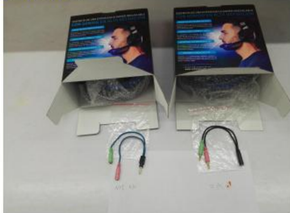
Wrong connection cable in package-Major
