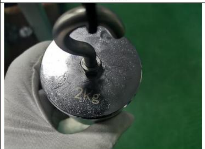
Cable pull test
