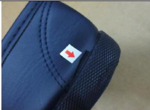
Outstanding flash at outsole ( Major Defect )
