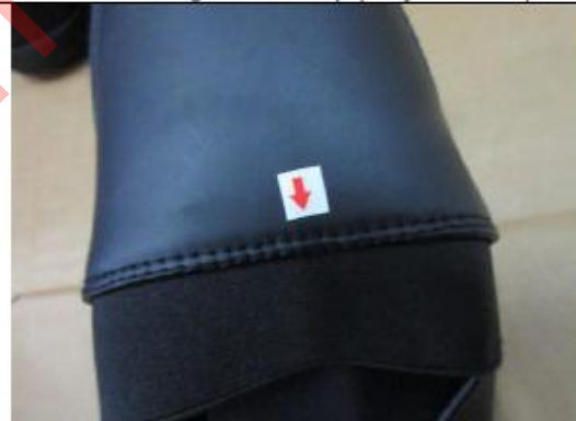
Outstanding Uneven Double stitches ( Major Defect )
