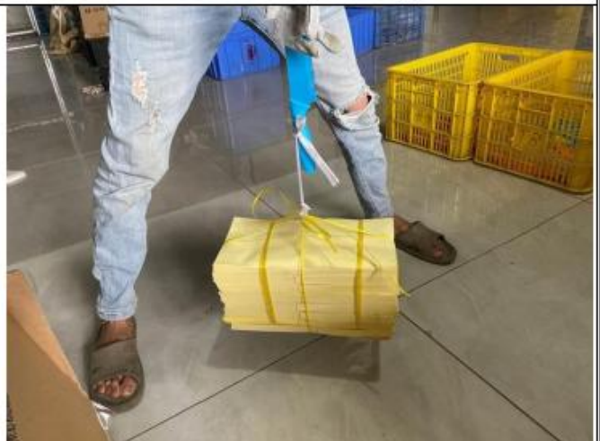
Abuse test with 6.75kgs
