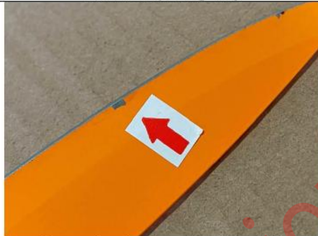
Poor coating / coating off on blade - Maj
