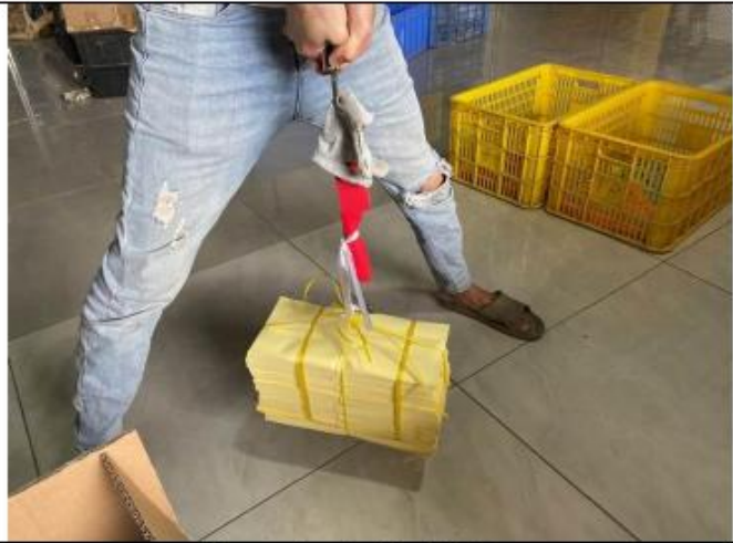
Abuse test with 6.75kgs
