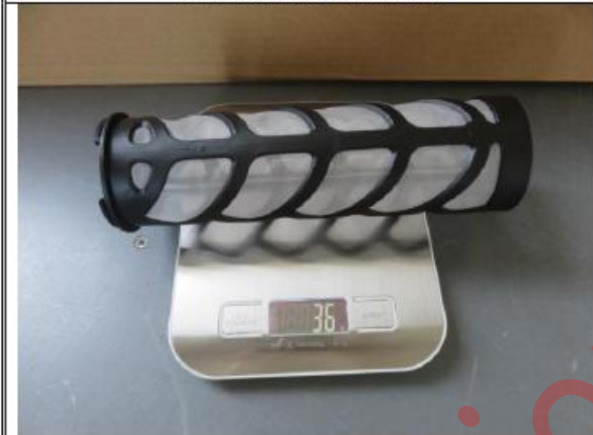
Infuser filter weight check
