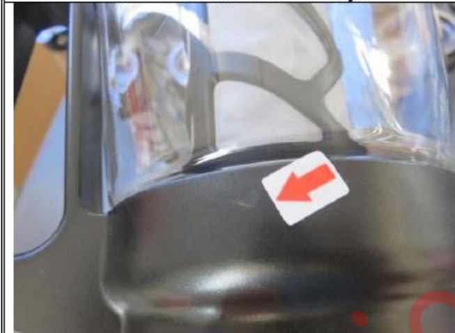
Dent mark on the surface-major
