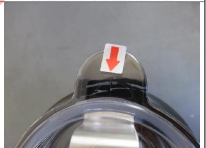
Scratches mark on the surface-minor
