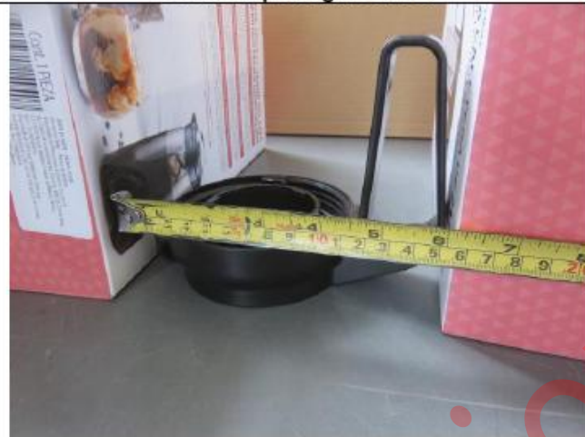
Handle and lid-filter support size check
