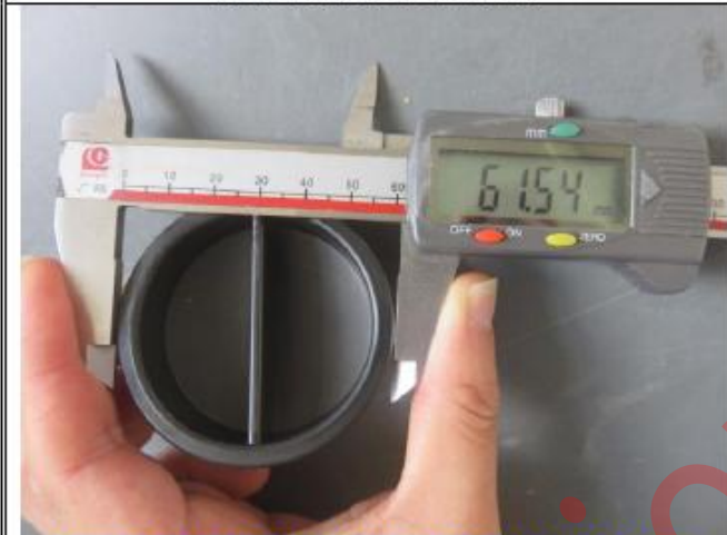
Cover for the infuser filter size check-61.54mm
