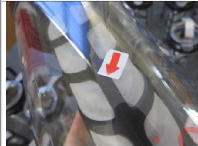
Scratches mark on the surface-minor
