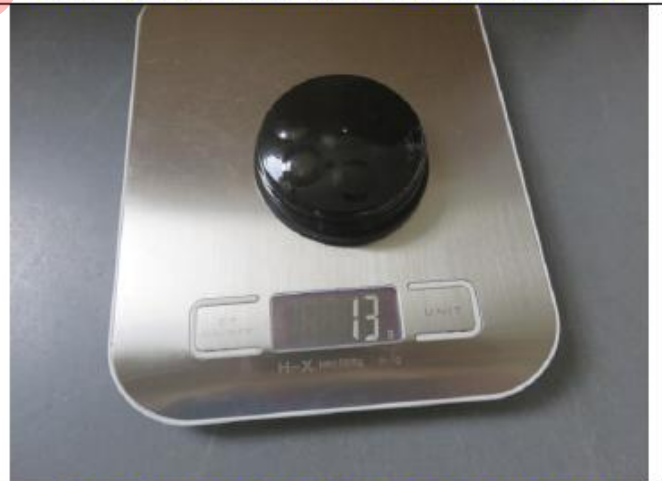
Cover for the infuser filter weight check-13g
