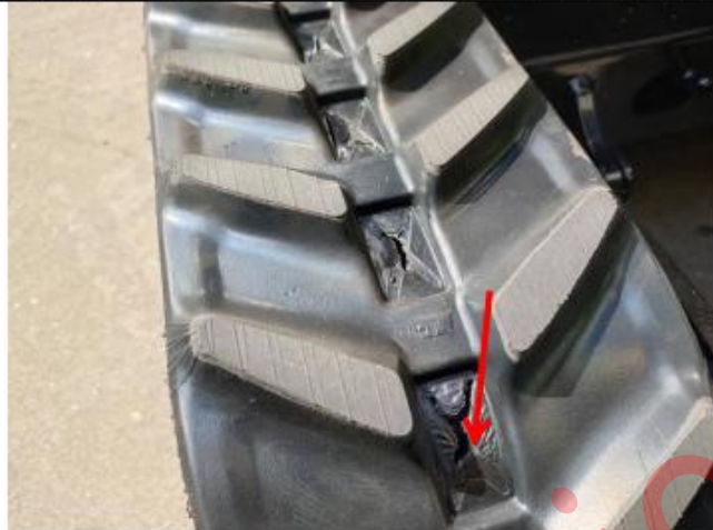
Remark 7. The weld line appearance is not look good. Pls refer to the picture.
