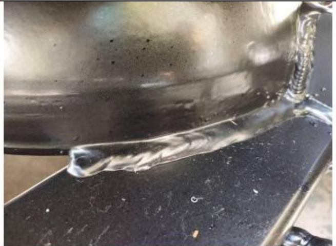
Remark 7. The weld line appearance is not look good. Pls refer to the picture.
