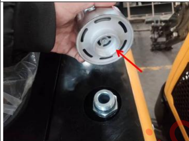
Remark 10. There are no oil seal on the tank cap.
