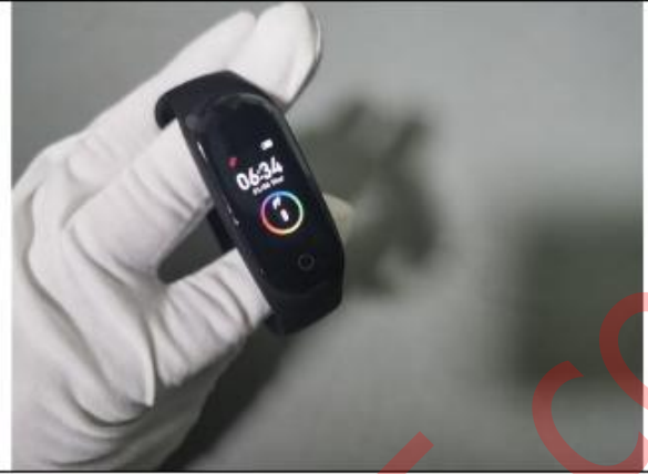
Bare drop test from 180cm
