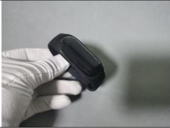
Bare drop test from 180cm
