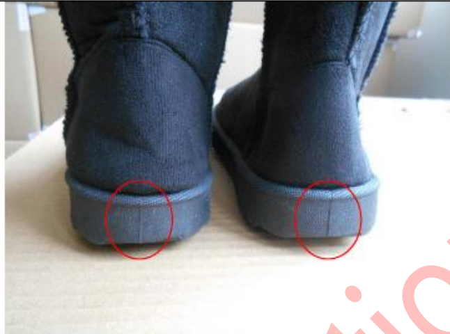
Remark 4: Actually found the trace of the mold at the heel of the outsole was obvious.
