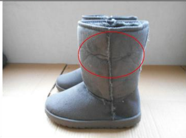
Remark 3: Actually found the upper surface of the product had slight crease due to the packaging method.
