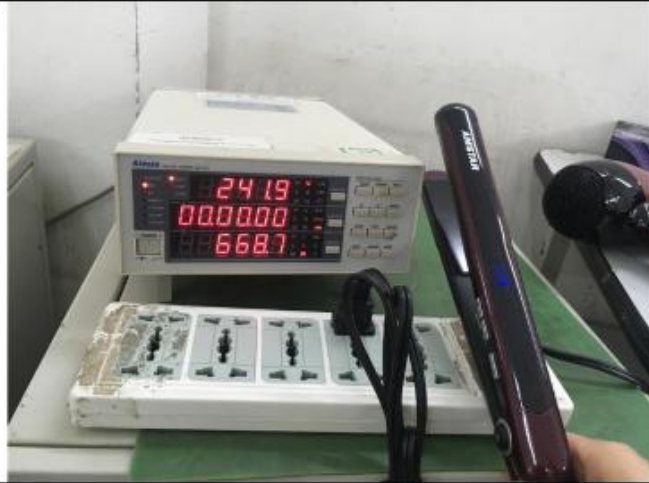
Blocked air inlet test for hair dryer
