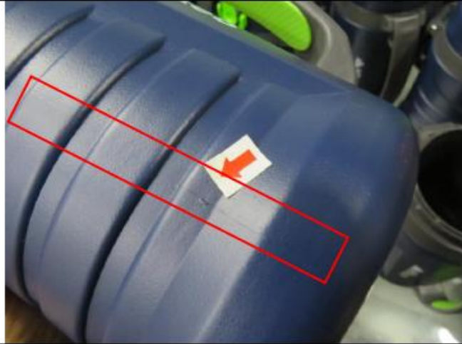
Remark 2: There were 100% of inspected samples with mold line on green button&bottle.
