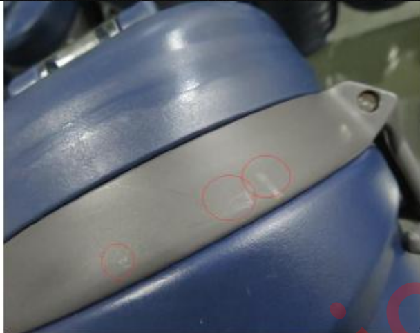
Remark 3: There were 100% of inspected samples with abrasion mark on surface.
