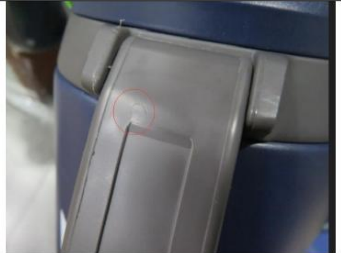
Remark 4: There were 70% of inspected samples with mold line on handle.
