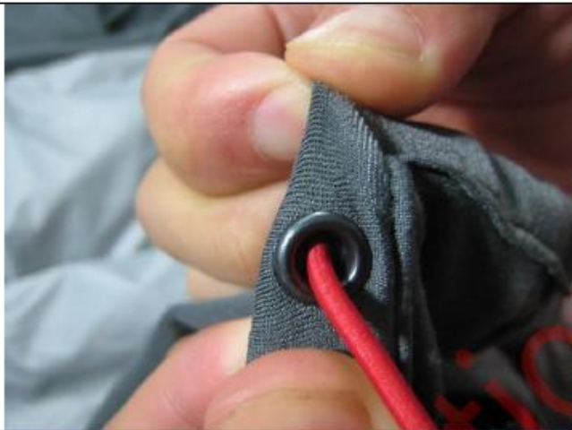
Pull test for fabric & eyelets, result is acceptable, OK
