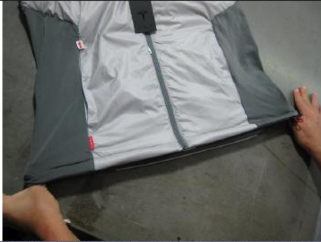
Stretching test for elastic cord & hem, result is acceptable, OK
