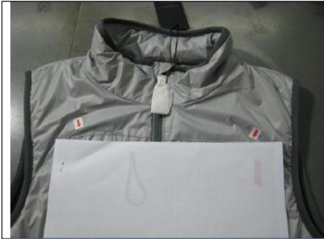
Mis-matched chest seam (right Vs left) (Major Defect)
