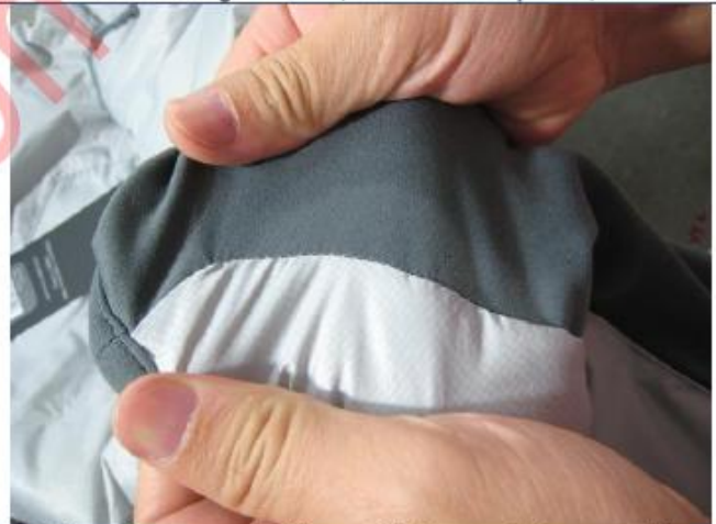
Pull test for seam of different fabric, result is acceptable, OK
