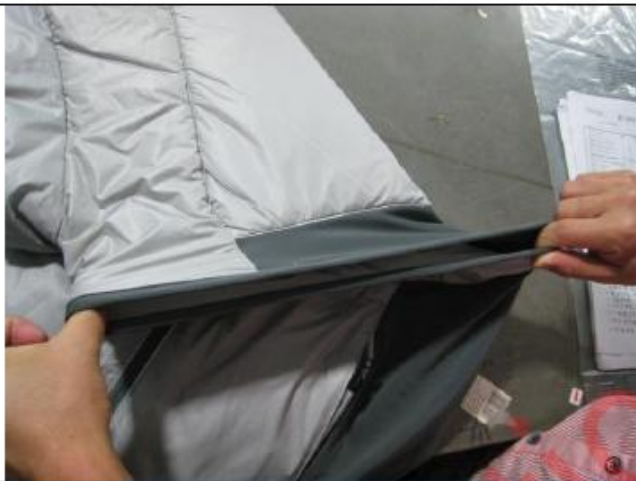
Stretching test for binding of armhole, result is acceptable, OK
