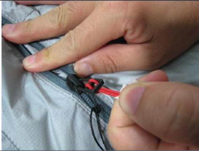
Pull test for red puller, result is acceptable, OK
