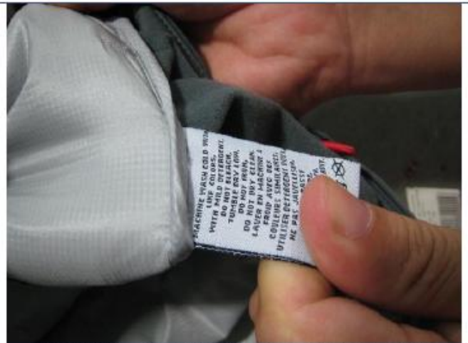
Pull test for composition & ware care label, result is acceptable, OK
