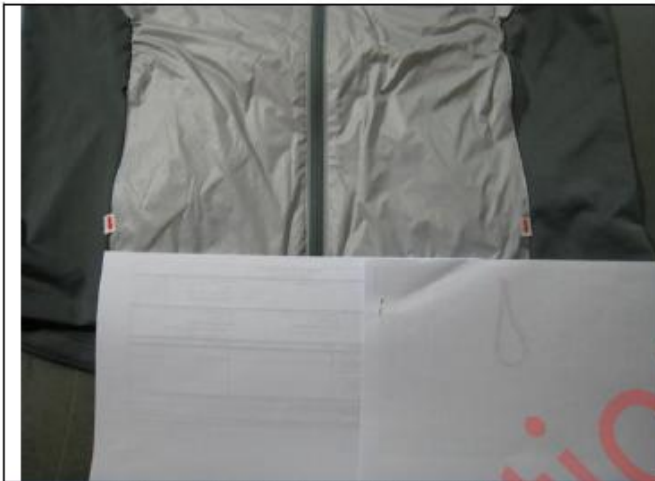
High-low tack (Right Vs left) (Major Defect)
