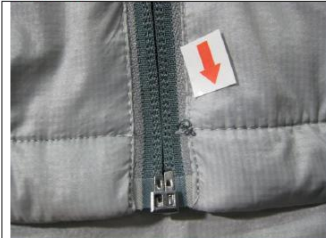
Mixed color of thread set in (Minor Defect)
