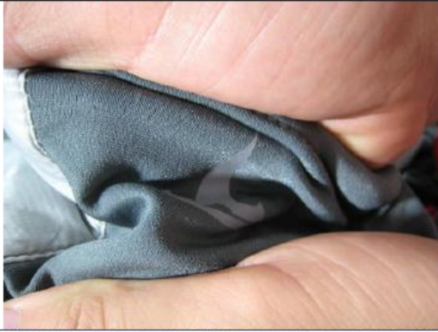
Rub test by hand for back T logo, result is acceptable, OK
