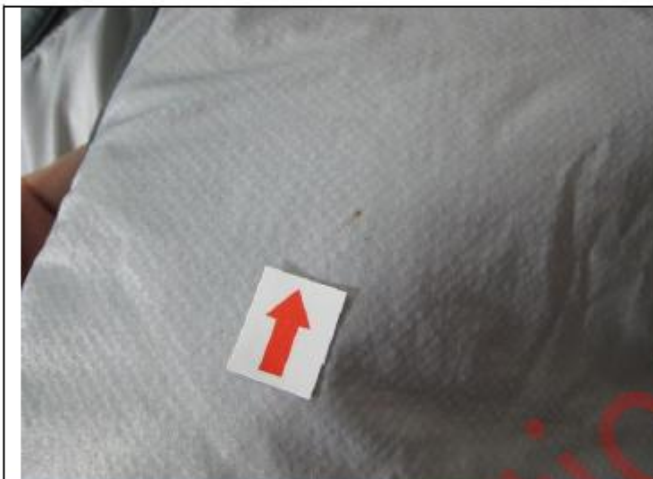
Dirt stain on fabric (Minor Defect)
