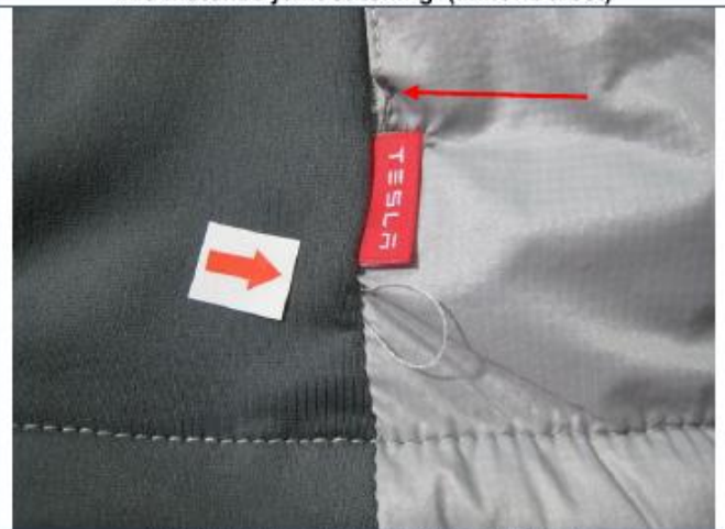
Visible bottom thread (Minor Defect)
