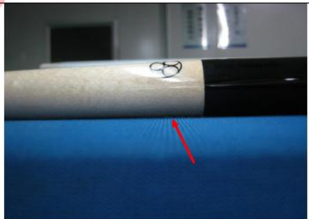
Wobble test after shaft installed with butt- other direction is wight slight gap, after rolling the cues
